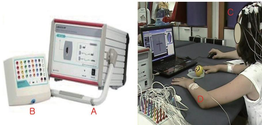
Fig. 1. The EEG set up. A: Main box; B: Junction box; C: 30 Ag-AgCl electrodes; D: 2 Electromyography electrodes. (Colours are visible in the online version of the article; <http://dx.doi.org/10.3233/NRE-2012-00803>)
